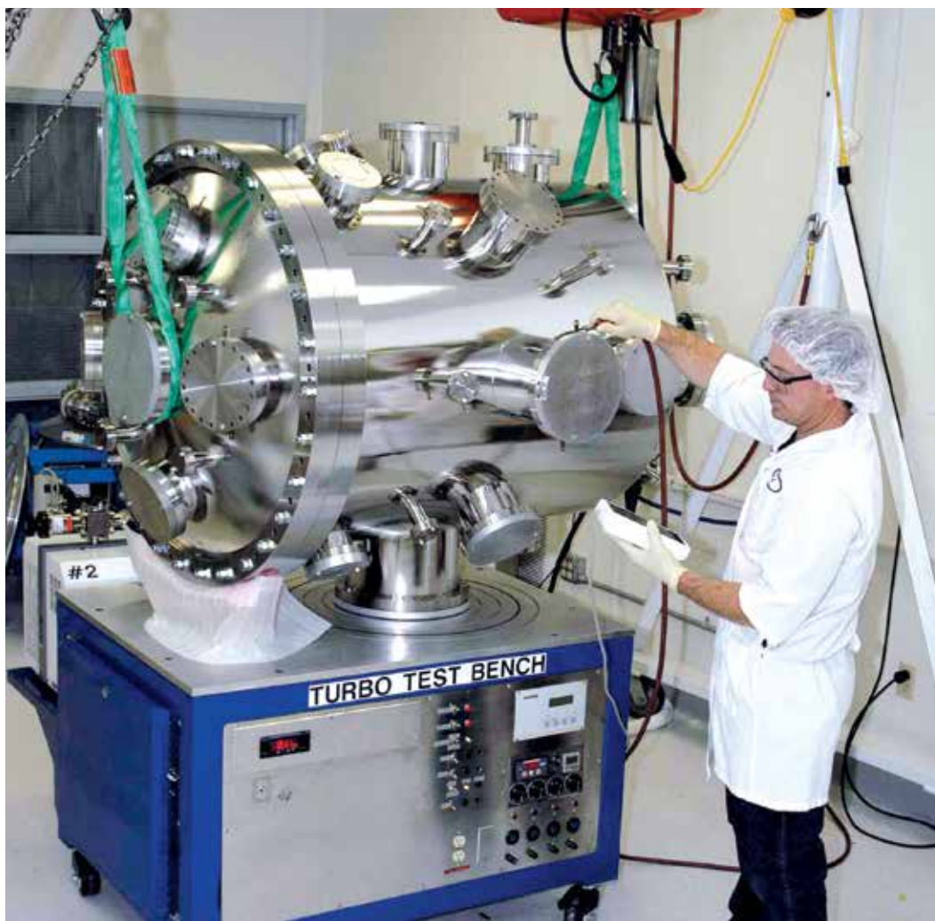
Chamber leak testing after mechanical inspection on chamber qualification test bench
