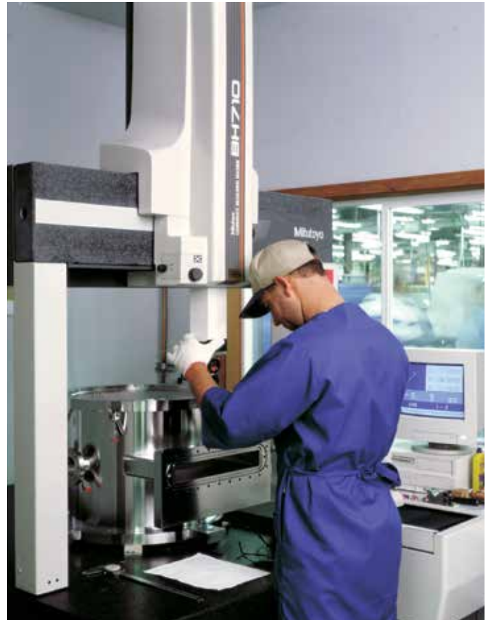
Mechanical inspection of process chamber with CMM
