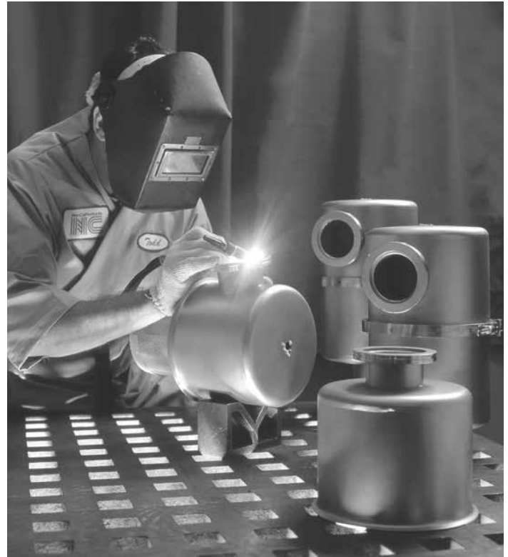
TIG Fusion Welding
