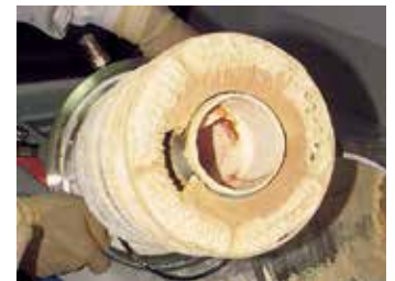
Water-cooled / particle trap for CVD
