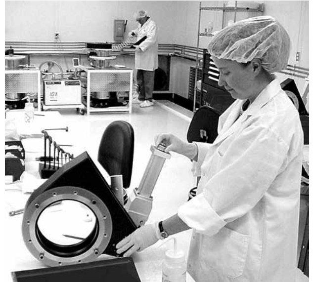
Heated pendulum valve assembly in our 3000 square foot Class 1000 clean room
