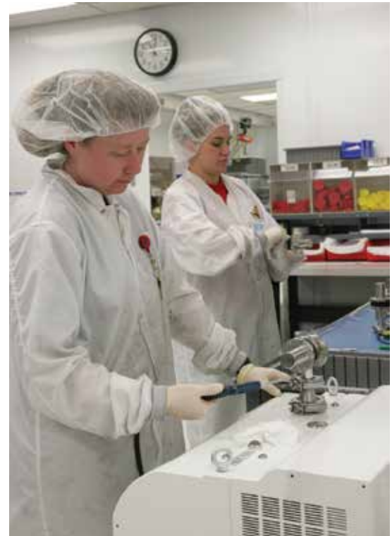
Dry leak detector for valve inspection
