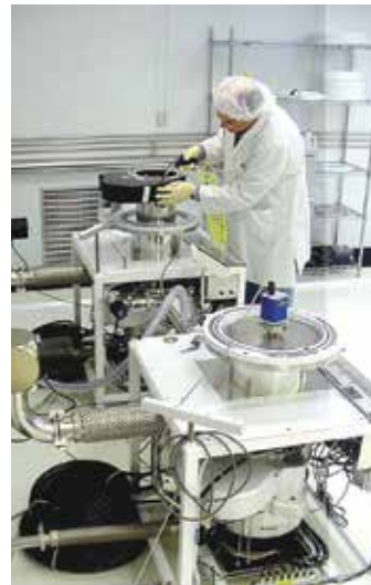
Leak testing pendulum valves
