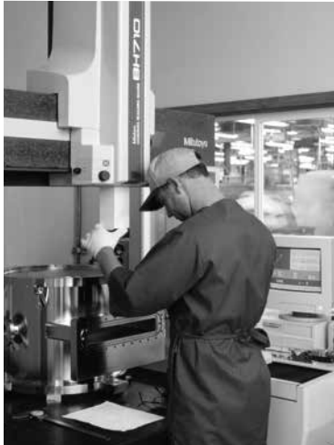
Mechanical inspection of process chamber with CMM (coordinate measuring machine)
