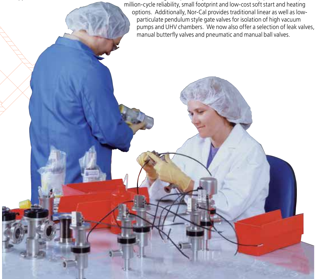
Valve assembly in Class 1000 clean room
